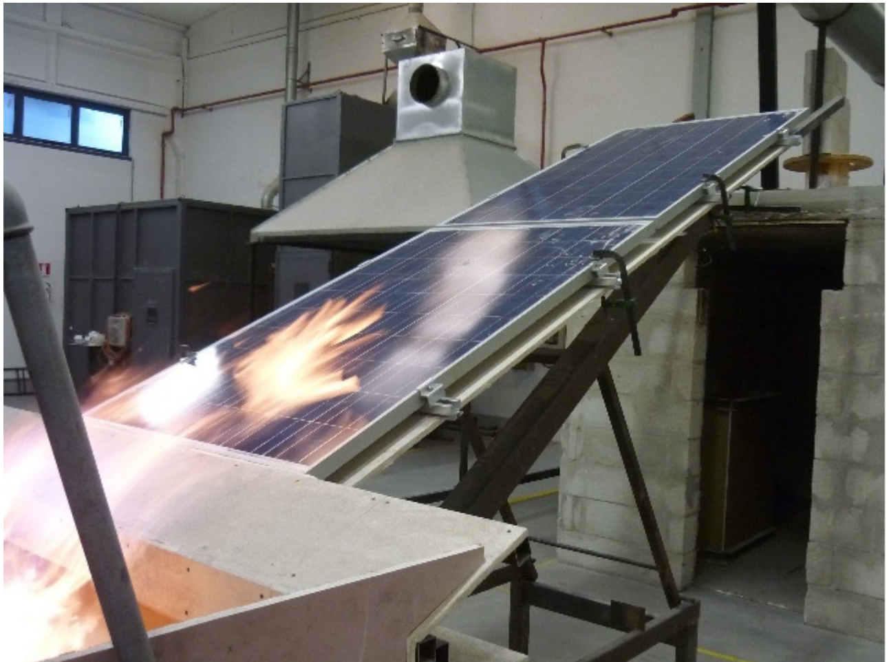
Figure 2 – Spread-of-flame test (LAPI laboratory)
